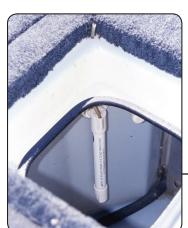
these systems can be easily improved by inserting a length of the appropriate-diameter aquarium air tubing into the vent hole on the top of the aspirator and routing the tubing to fresh air.
